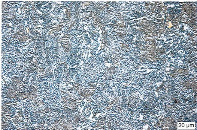
The fine grain treatment for 20MnCrMo7 steel is achieved by alloying niobium (columbium) and titanium during melting. This, however, leads to sporadic precipitations of titanium carbonitrides of max. 25 µm, as can be seen in Fig. 6.
